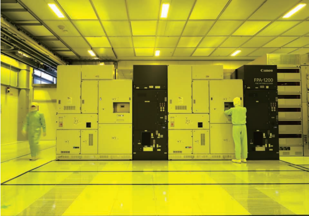
Nanoimprint semiconductor manufacturing equipment aimed at mass production of semiconductor devices
